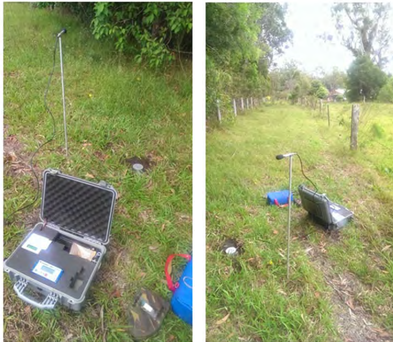
Figure 11 InstanTel® Minimate Plus™ vibration monitor and geophone
